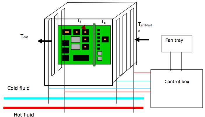
Figure 2. Hypothetical Schematic of an Adaptive System for a Server.
